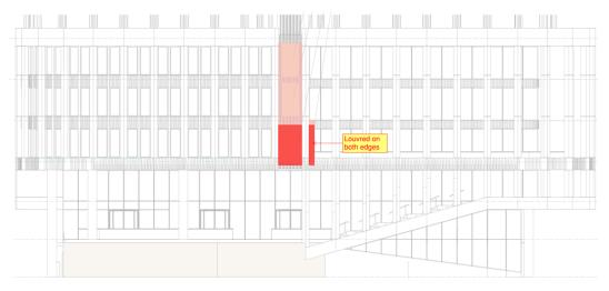
Figure 5 – Location of proposed Kitchen exhaust louvres (East Elevation)
