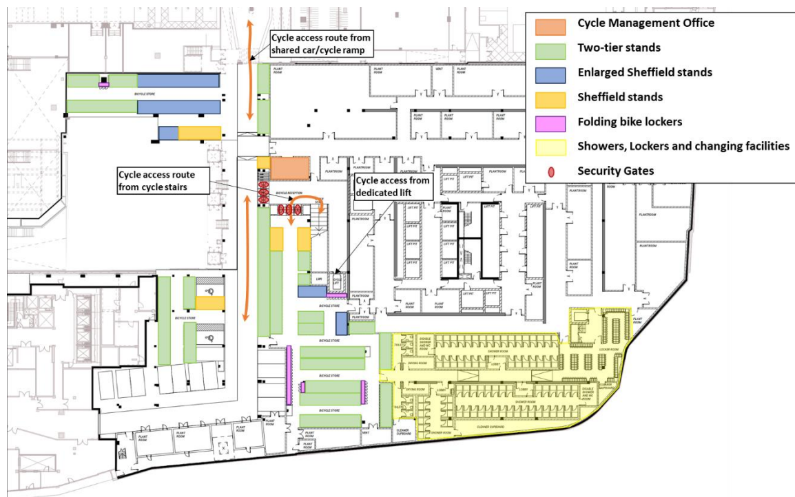
Figure 4-11: Proposed Cycle Parking Layout – Basement
