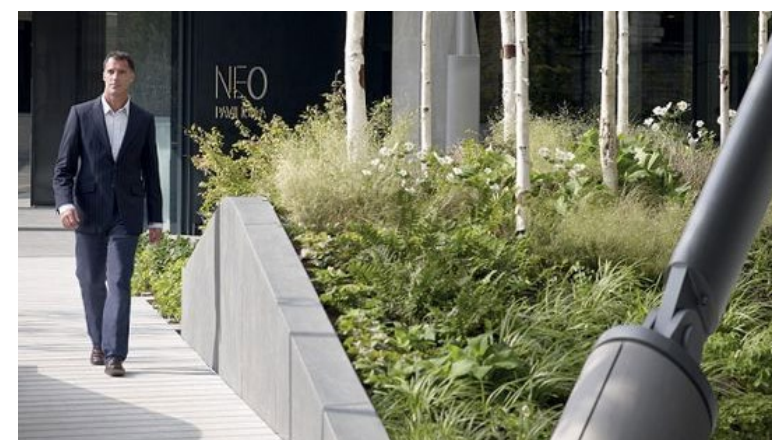
02 Throughout the design, large mounds shape the landscape, offering additional security support through their height and immovability. These planters will have an external planter wall height of min. 650mm.
