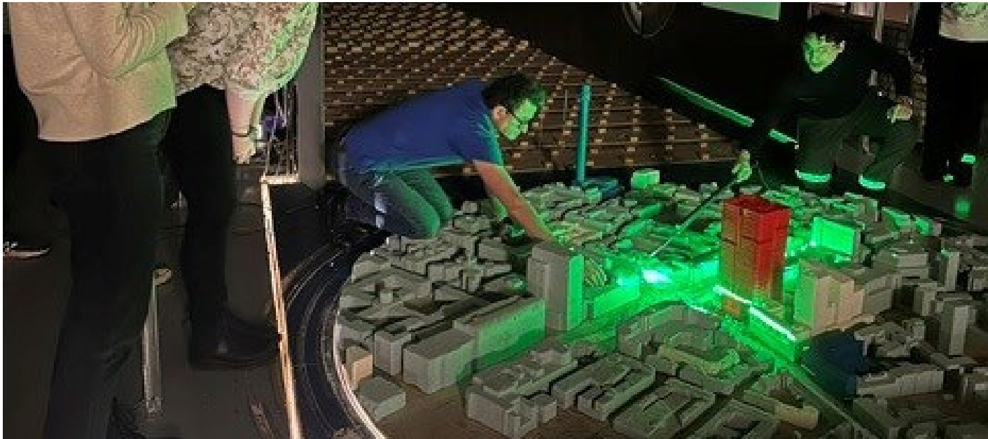
Massing model and sensors used for wind tunnel testing
