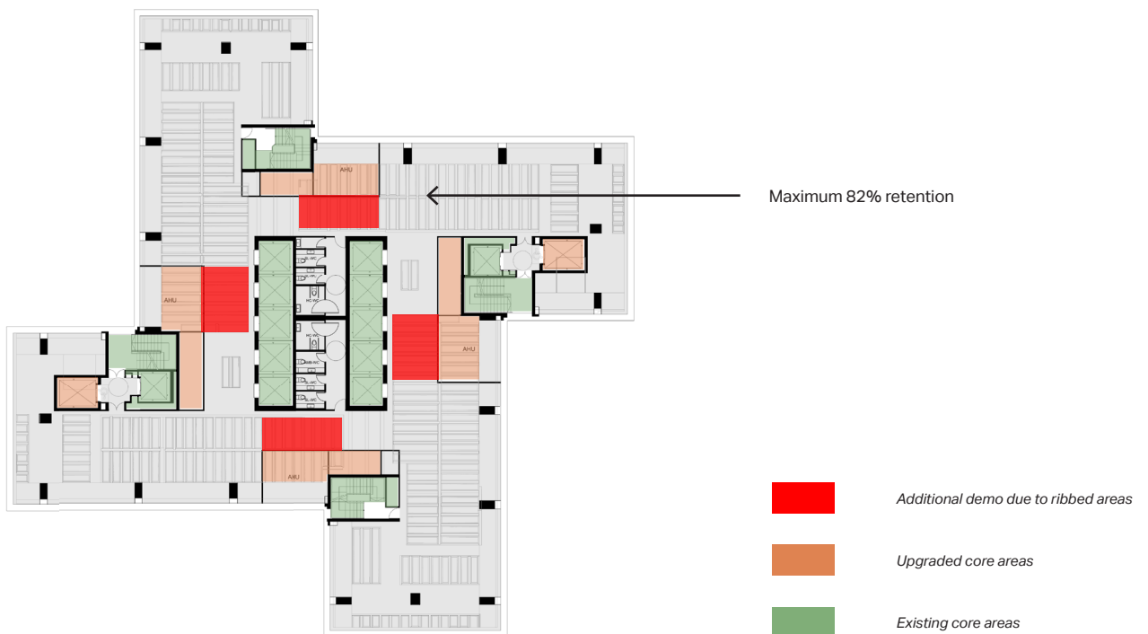
Figure 15.2 Diagram showing erosion of floor slab due to upgrades to meet current Building Regulations
