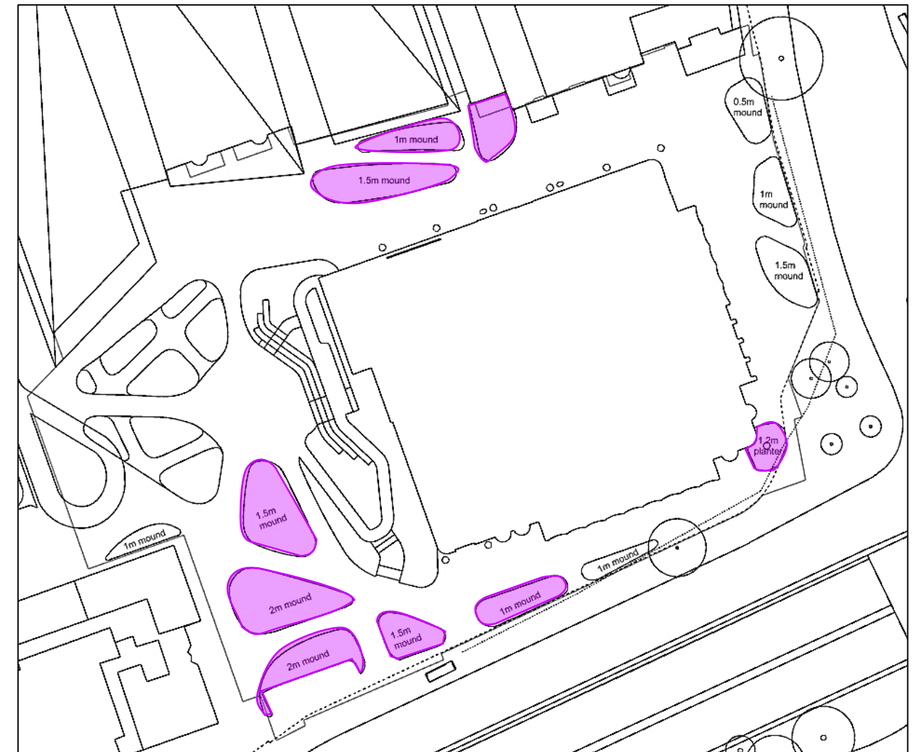
Figure 11.31 Plan of the Amended Proposed Development with Mound Heights of the Landscaping 6
