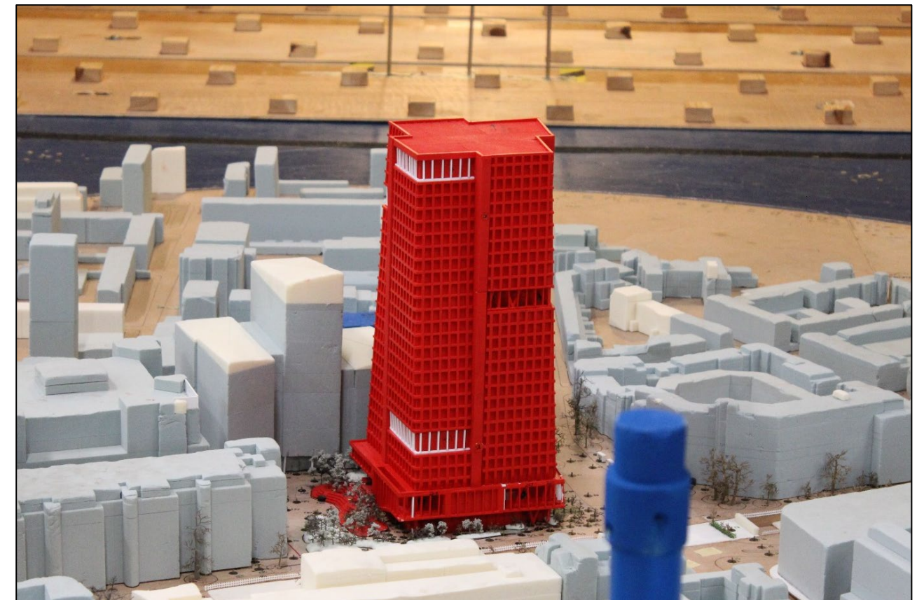
Figure 11.23 Photos of the Model Used in the Wind Tunnel for Configuration 3a: Proposed Development with Landscaping and Initial Mitigation Model
