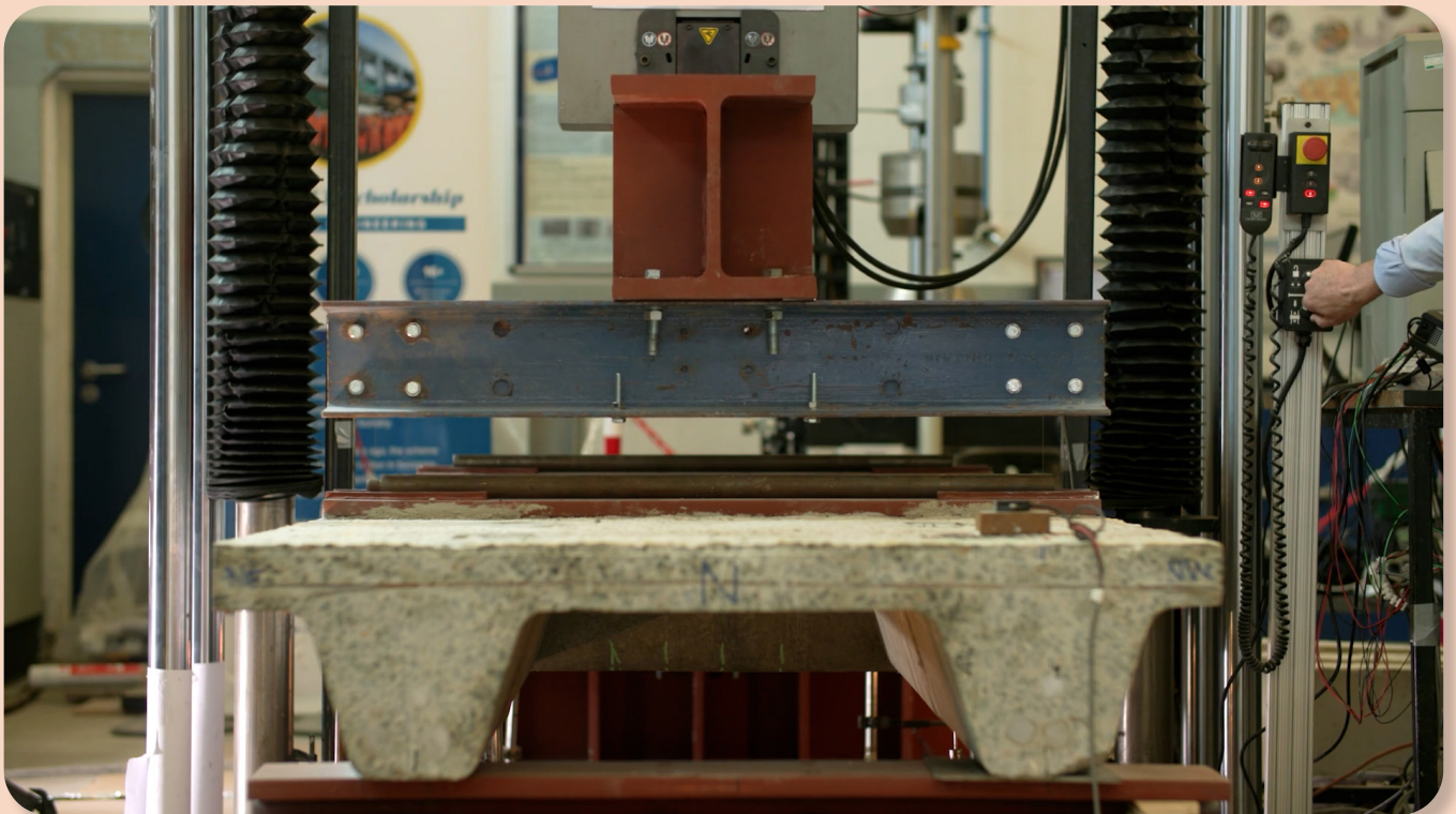
Figure 3.13 Image showing the slab specimen in the testing rig at the University of Surrey.
