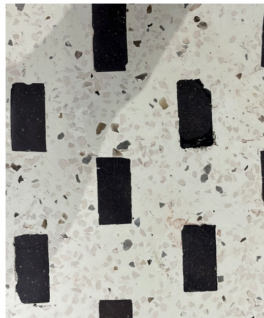
Figure 4.29 Trial terrazzo made using inert material from Euston Tower
