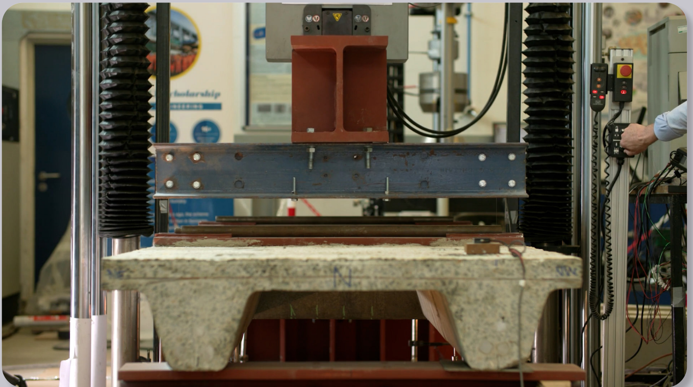
Figure 2.21 Image showing the slab specimen in the testing rig at the University of Surrey.
