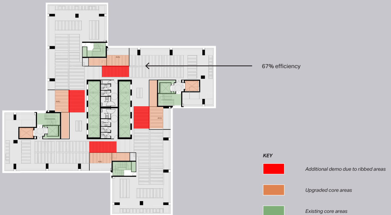
Figure 2.5 Diagram showing erosion of floor slab and exaggerated penetrations due to upgrades to meet current Building Regulations
