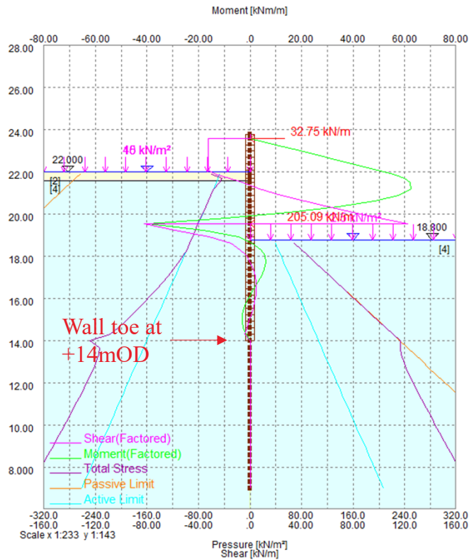
STAGE 11 : Concrete relaxation Results for factor set Eurocode 7 (UK - BS EN 1997-1:2011) DA1-2
