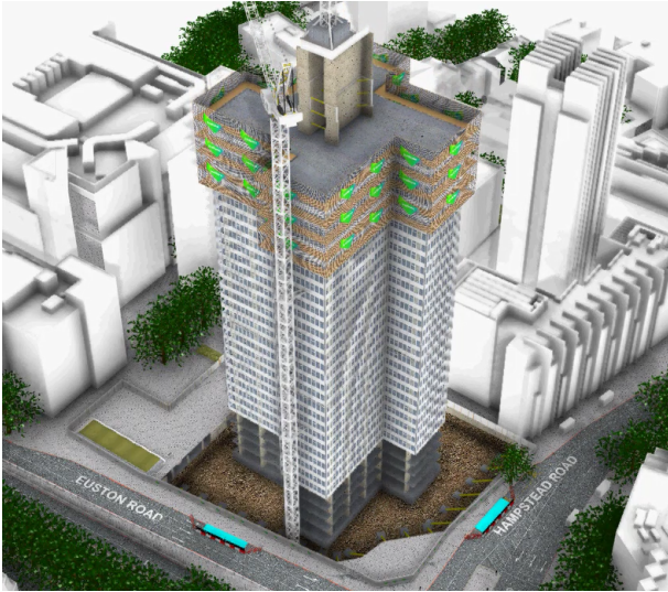
a) Deconstruction of floorplates starting from roof level downwards. Removal of ground floor slab and installation of temporary props to support the basement wall.
