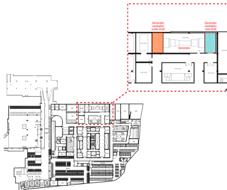
Figure 10 – Image showing the generator plantroom location in the basement of Euston Tower
