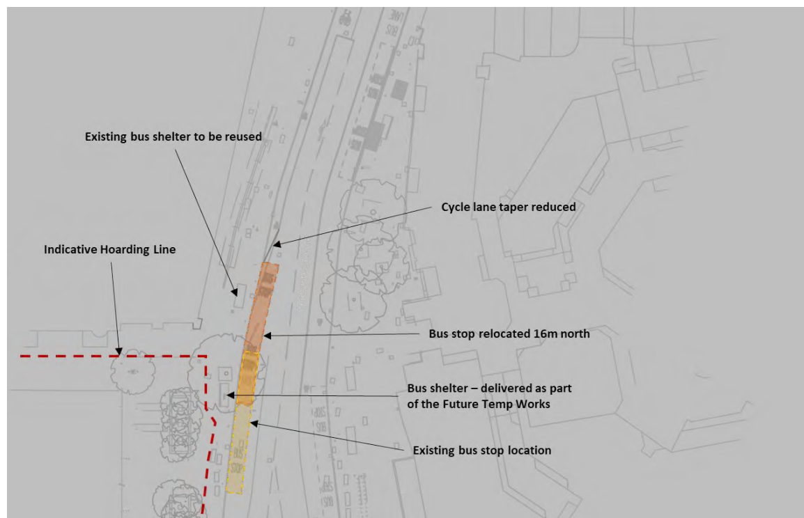
Figure 8-24: Proposed Hampstead Road Bus Stop Relocation
