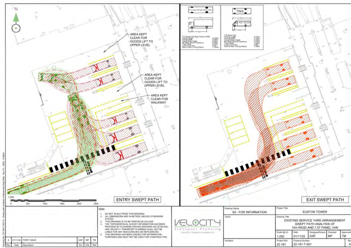
Figure 4-10: Existing Service Area - Swept Path Analysis
