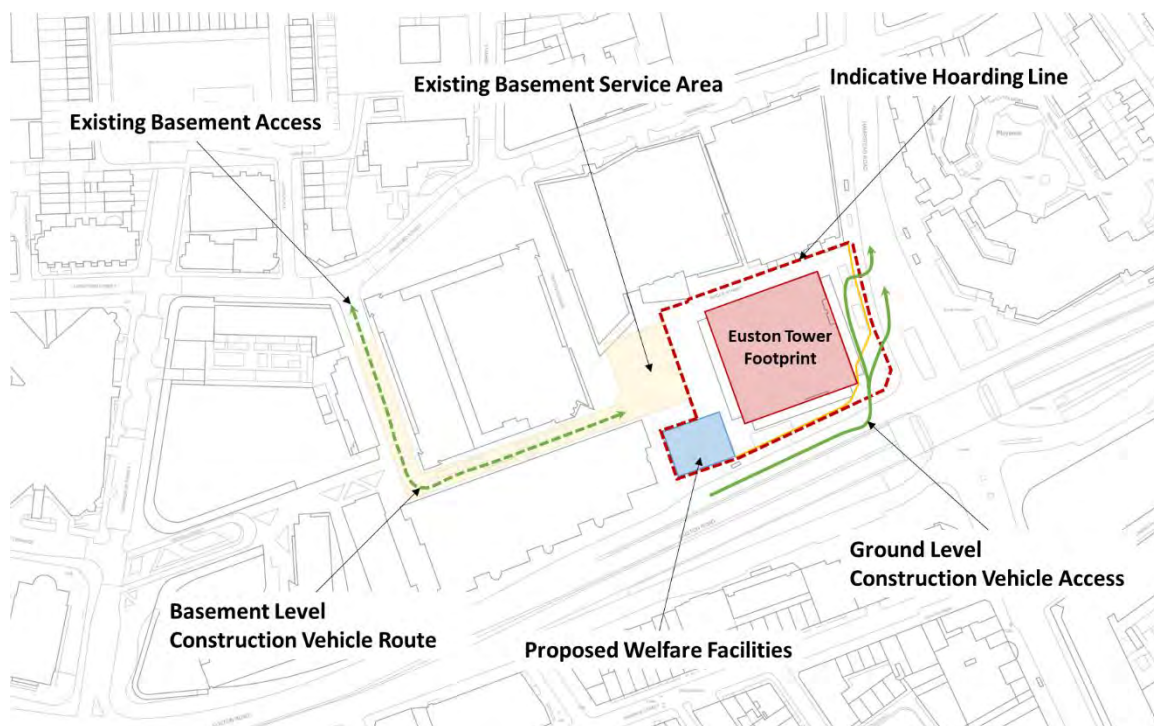
Figure 8-31: Indicative Construction Logistics Strategy
