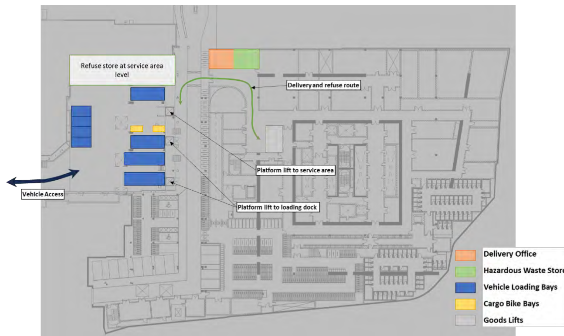
Figure 5-3: Proposed Basement Servicing Arrangements
