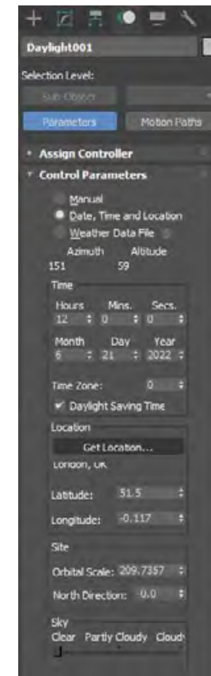
Figure E.22: Screenshot of environment information (time, date and year) entered to locate the sun correctly (see Section 7).
