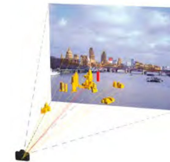
Figure E.17: The camera matched background plate with an example of a proposed scheme included in red
