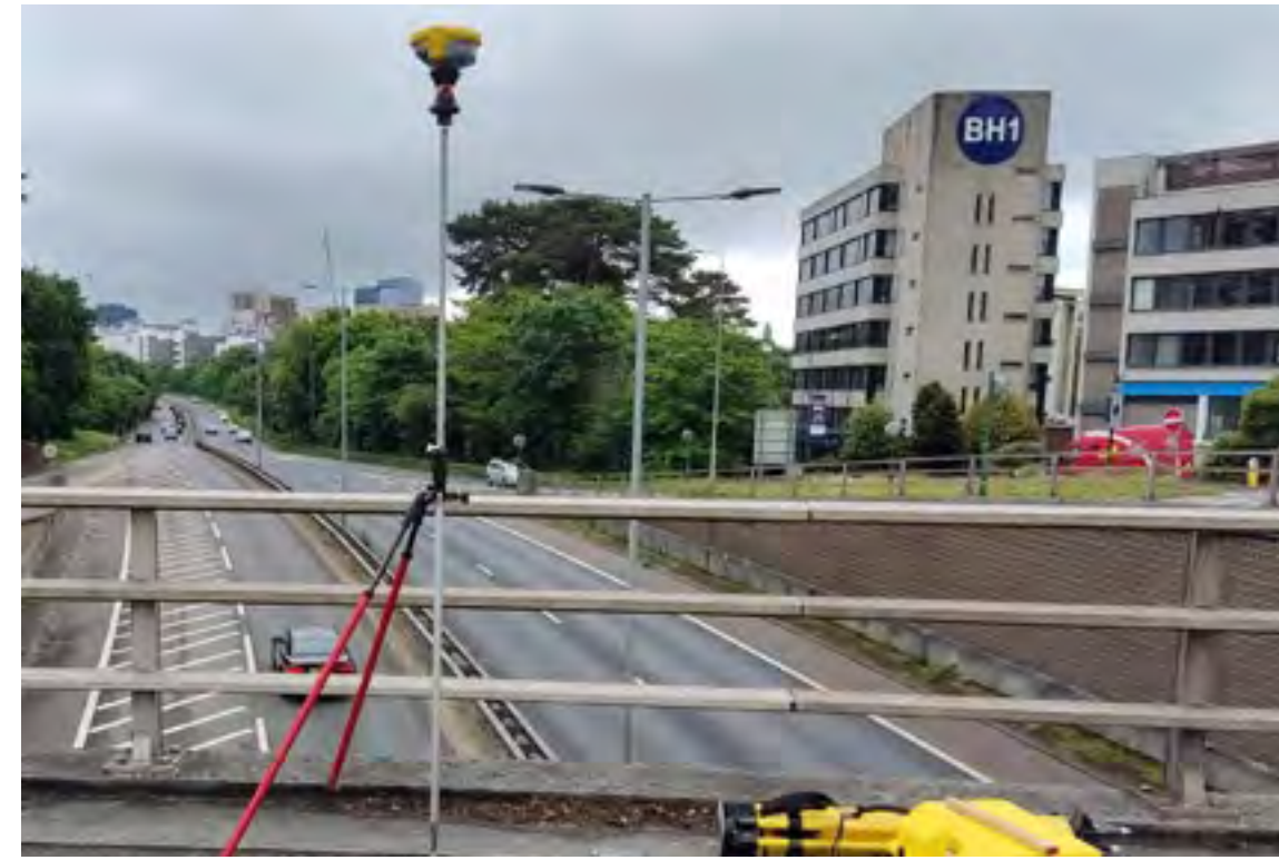
Figure E.7: Field survey being carried out, GNSS receiver
