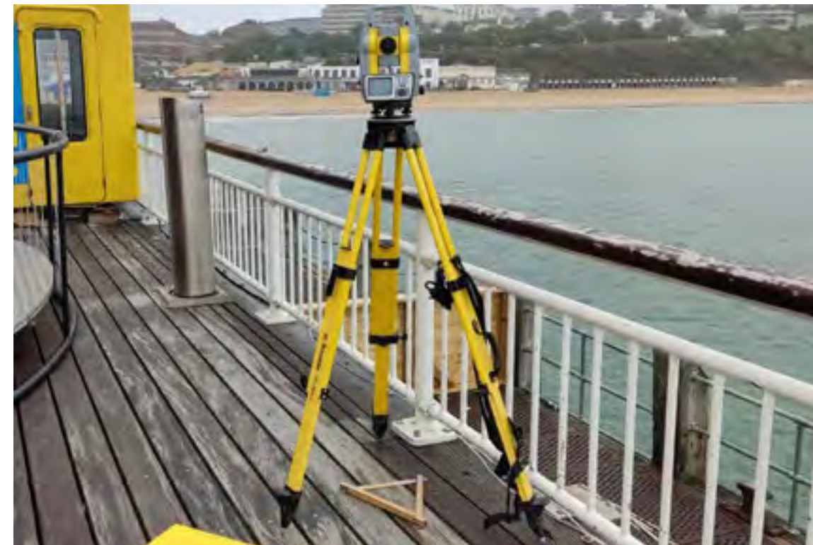
Figure E.8: Field survey being carried out, total station
