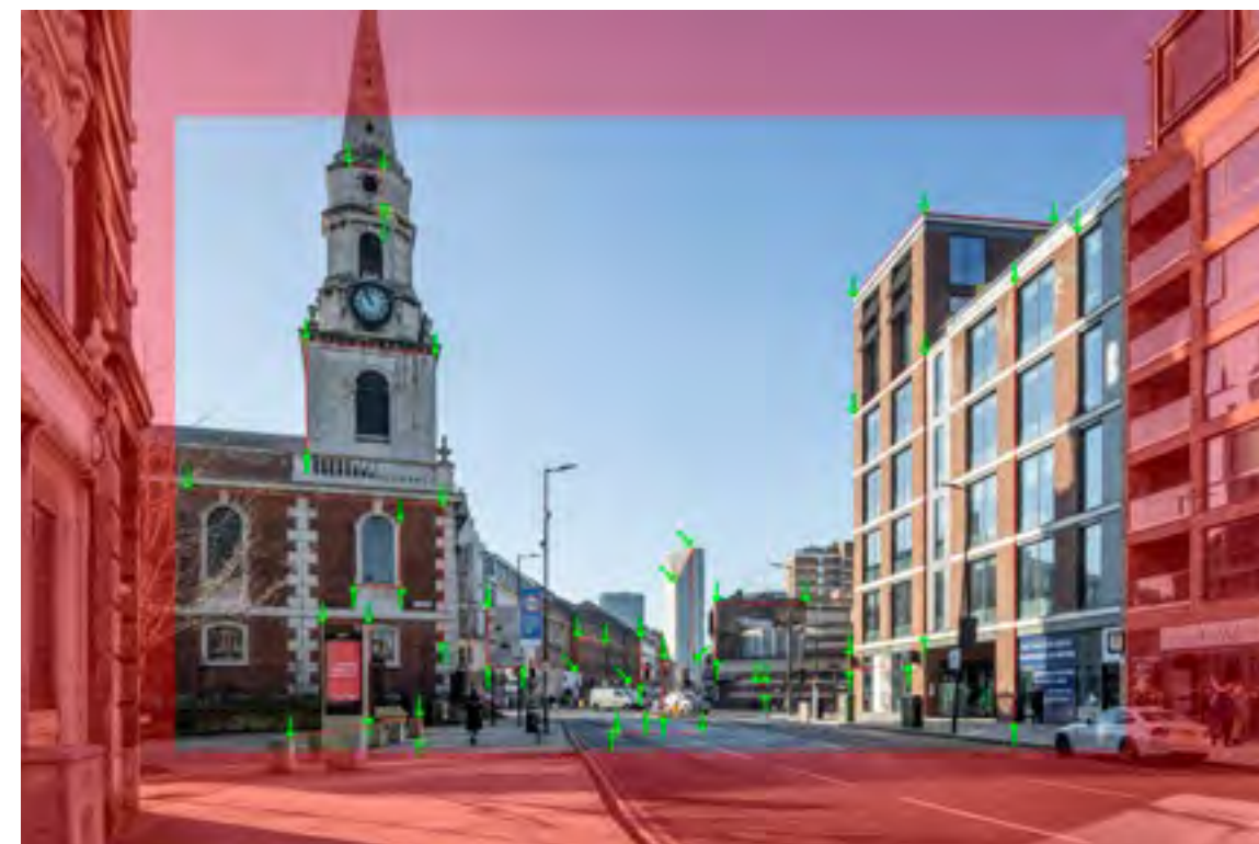
Figure E. 6: Background plate highlighting critical survey points in green and secondary survey strings in red
