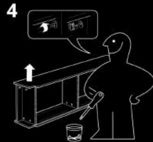
4 Place on side and remove screws.
