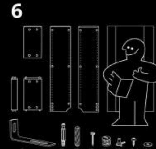
6 Here are all the parts you should have for your disassembled BILLY.
