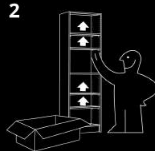
2 Remove shelves, shelf support pins and wall brackets.
