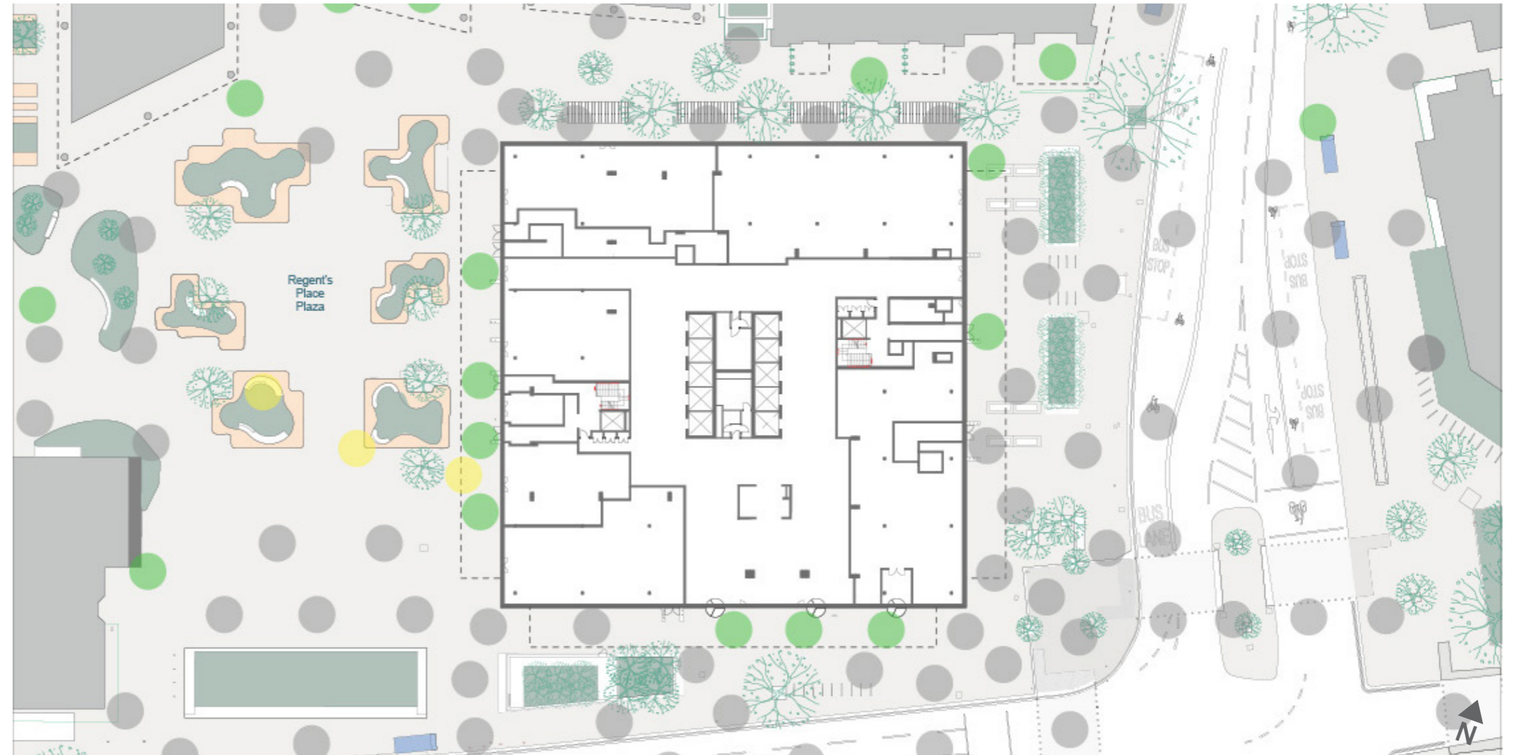
Site Plan of maximum tolerable wind conditions (worst case - winter). Adapted from figure 11.2 in ES Volume 1, Chapter 11. Refer to ES for further details on wind conditions.
