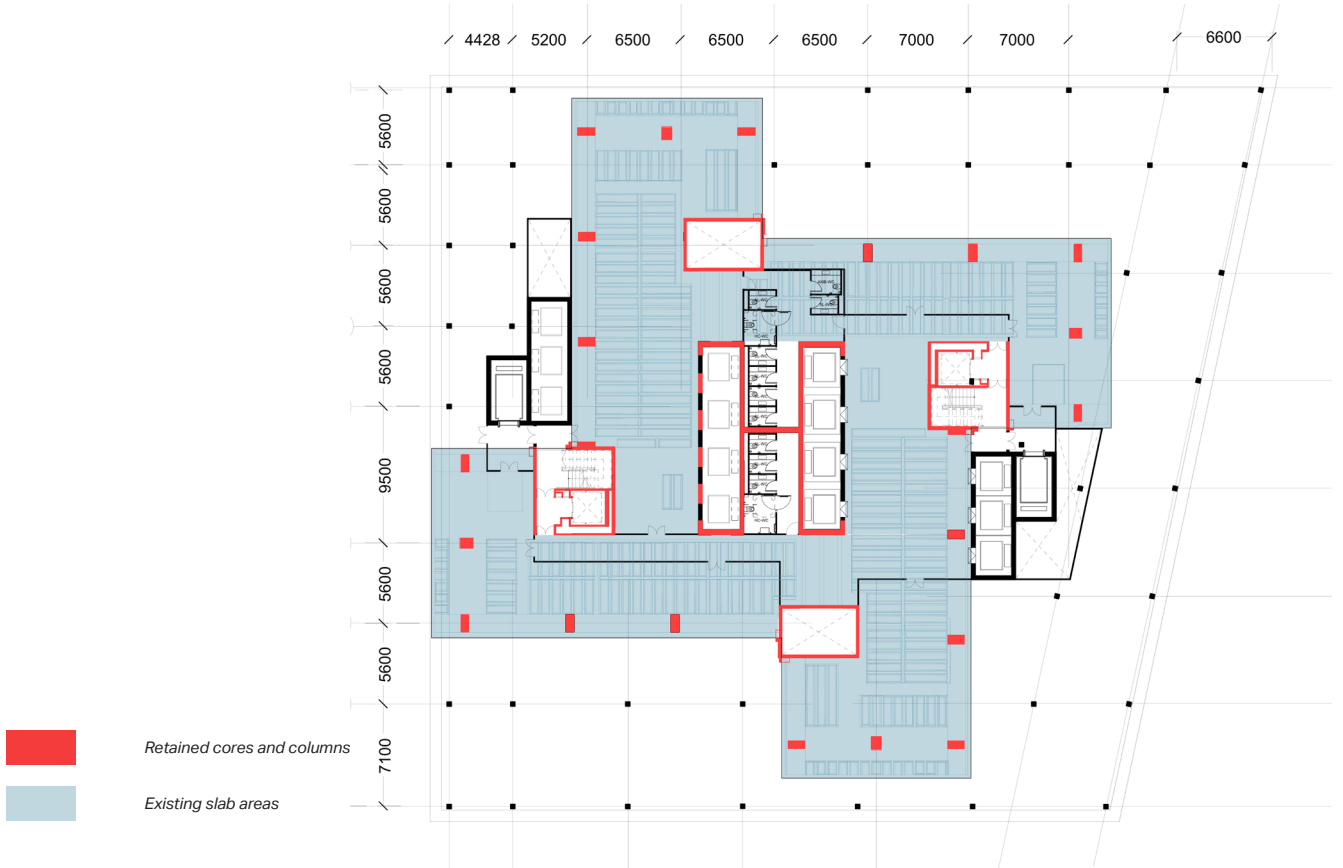
Figure B.3 Structural overlay showing the extent of existing slab and structure retained with dispersed core layout
