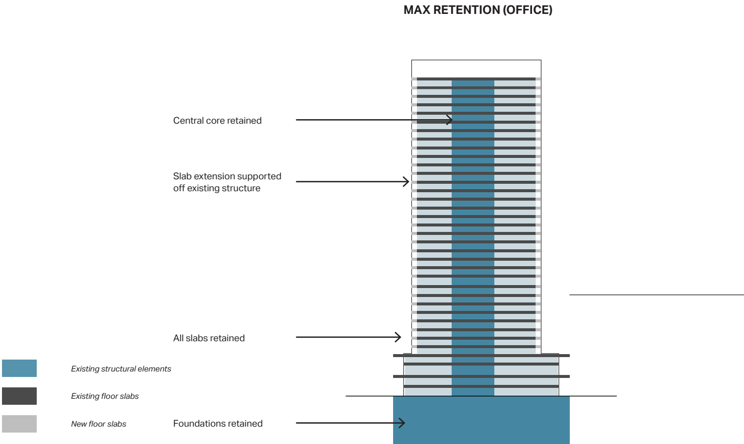
Figure 16.5 Diagram showing retained structural elements in this option (section above and slabs opposite)
