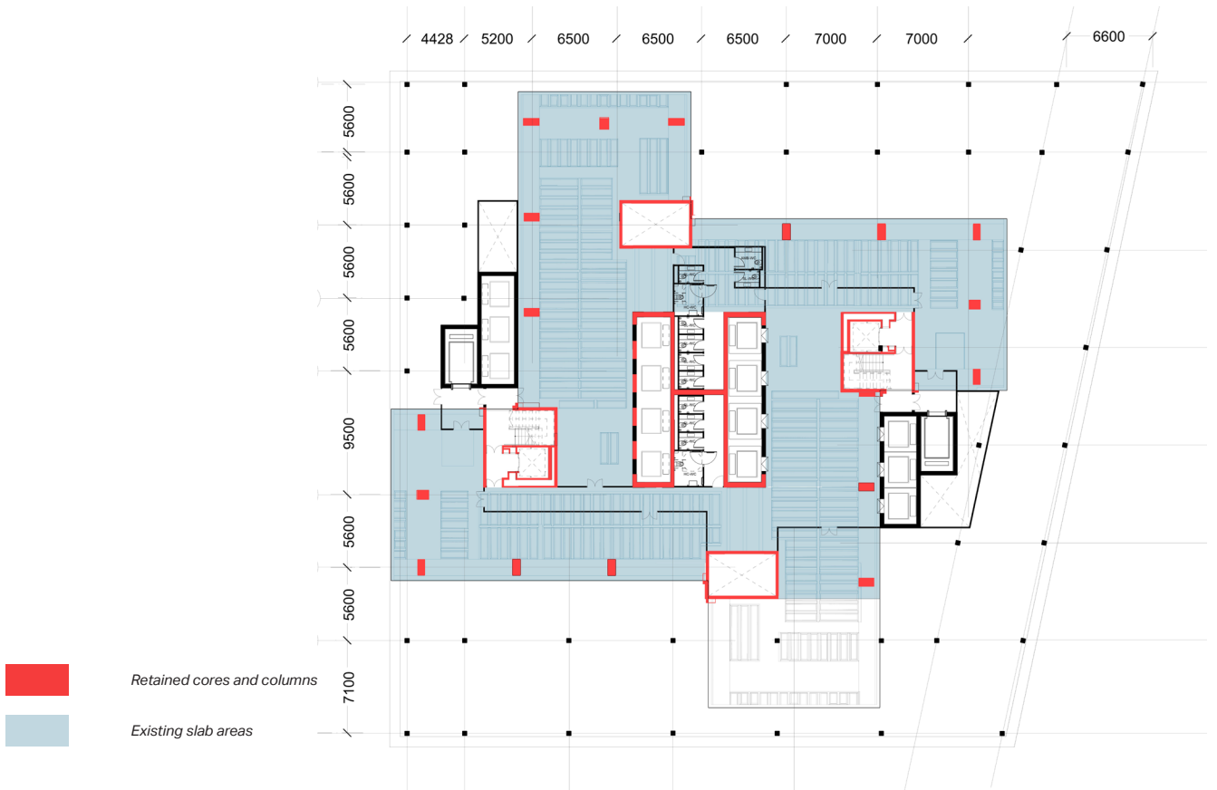
Figure B.5 Structural overlay showing the extent of existing slab and structure retained with dispersed core layout
