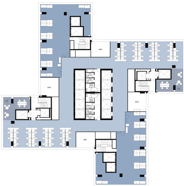
Figure 10.6 Typical tower level lab-enabled test-fit for lower portion of stack. One lift bank doesn't open on to the lab floors.
