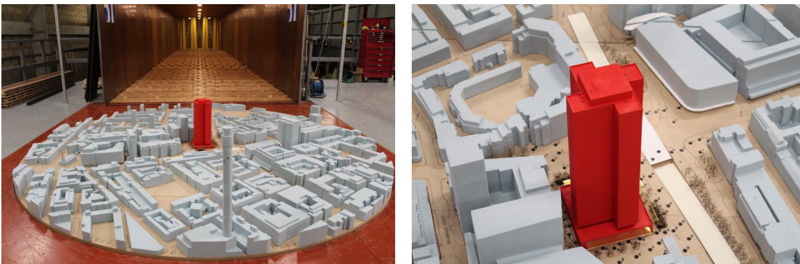
Figure 10.26 Wind tunnel models for the existing tower
