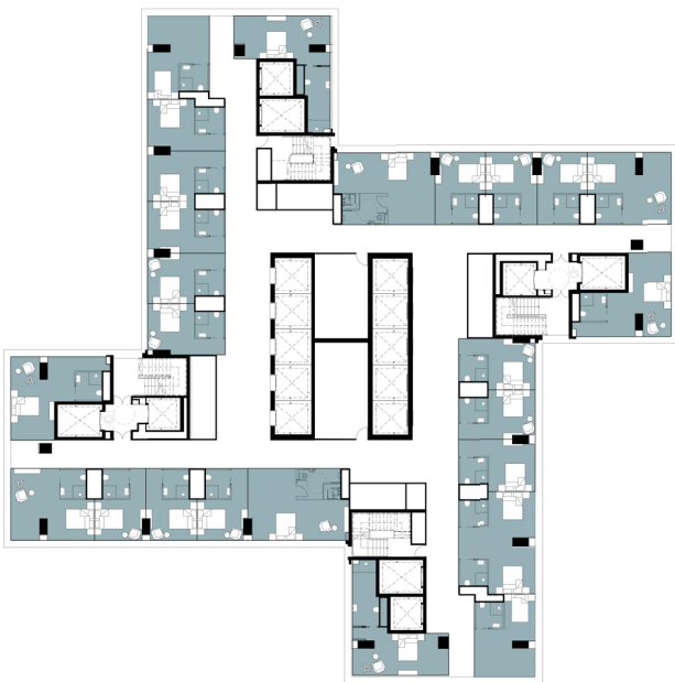
Figure 11.3 Typical floorplates for hotel floors in hotel and student accommodation scenario. One lift bank doesn't open on to the student accommodation floors.
