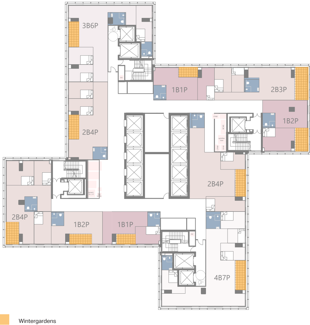
Figure 10.28 Typical tower level residential use test-fit. Market rate mix with private amenity (winter gardens highlighted)
