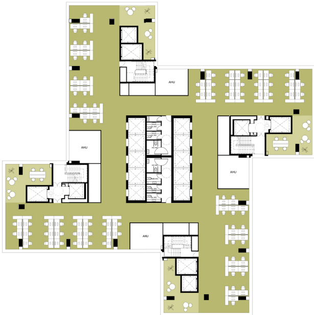
Figure 10.4 Typical tower level office test-fit for lower portion of stack. One lift bank doesn't open on to the office floors.
