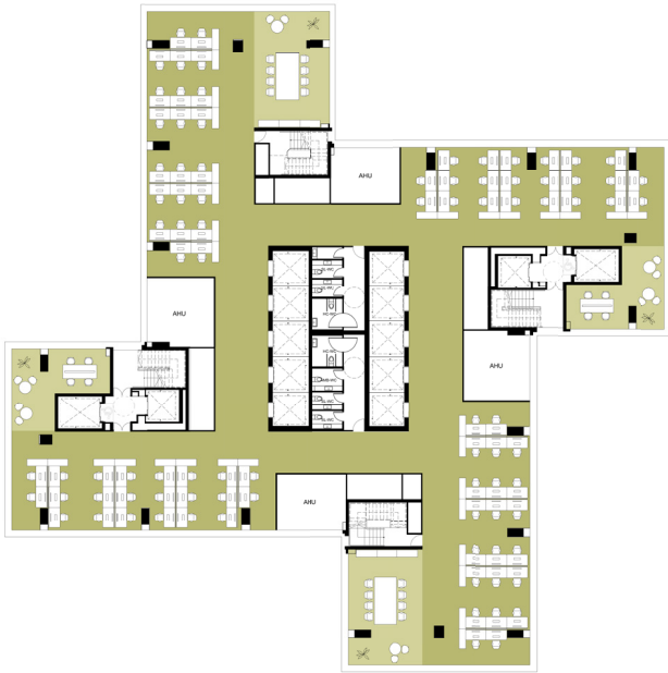
Figure 9.2 Typical floorplates for offices in office-only scenario with 4 no. AHUs per level
