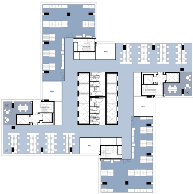
Figure 9.3 Typical floorplates for labs in office and lab-enabled scenario with 4 no. AHUs per level.
