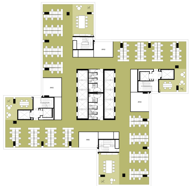
Figure 9.4 Typical floorplates for offices in office and lab scenario with 4 no. AHUs per level.
