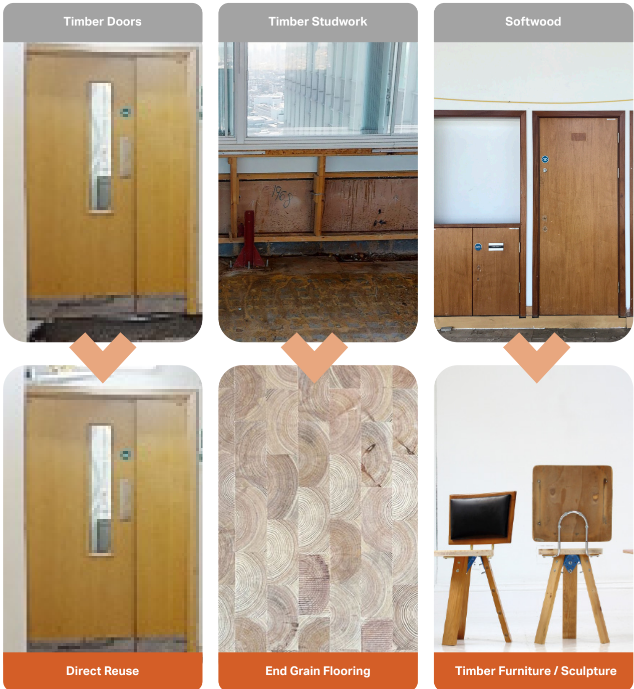
Figure 4.34 Sketch ideas for either direct reuse or remanufacturing of existing timber elements
