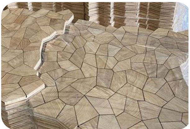
Figure 4.35 Process for remanufacturing timber into flooring (above) and reference images of end grain timber products (below)
