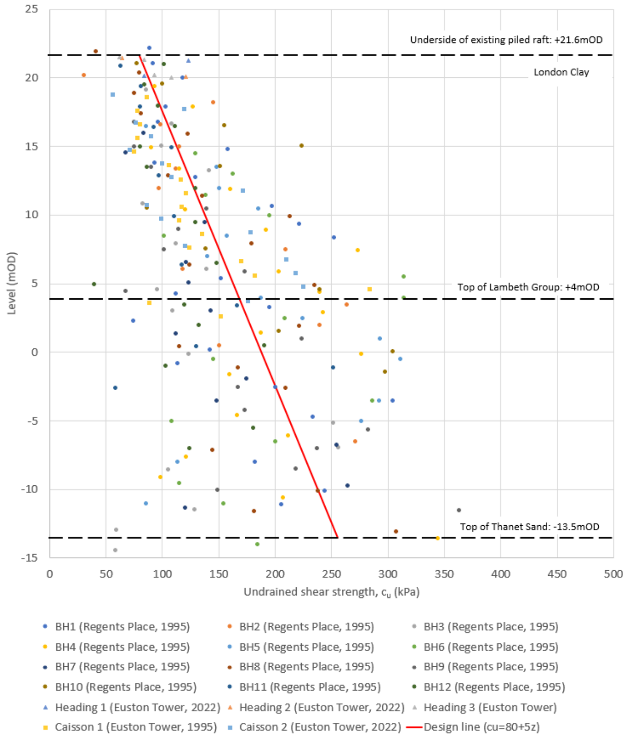
Figure 15: Undrained shear strength from Undrained Unconsolidated triaxial results on 100mm diameter samples.
