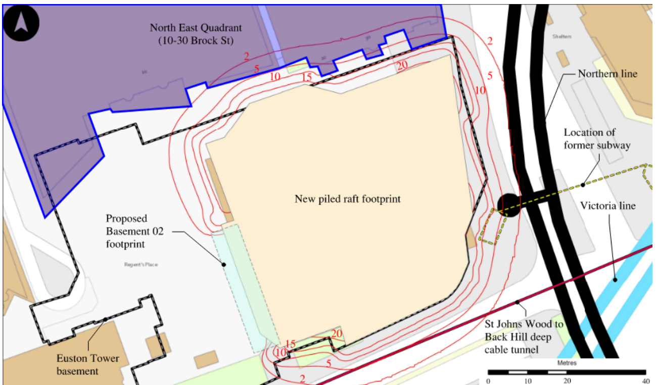
Figure 26: Calculated long term settlement (mm) at basement level +21.6mOD resulting from partial superstructure deconstruction, proposed Basement 02 excavation, and new superstructure loading.
