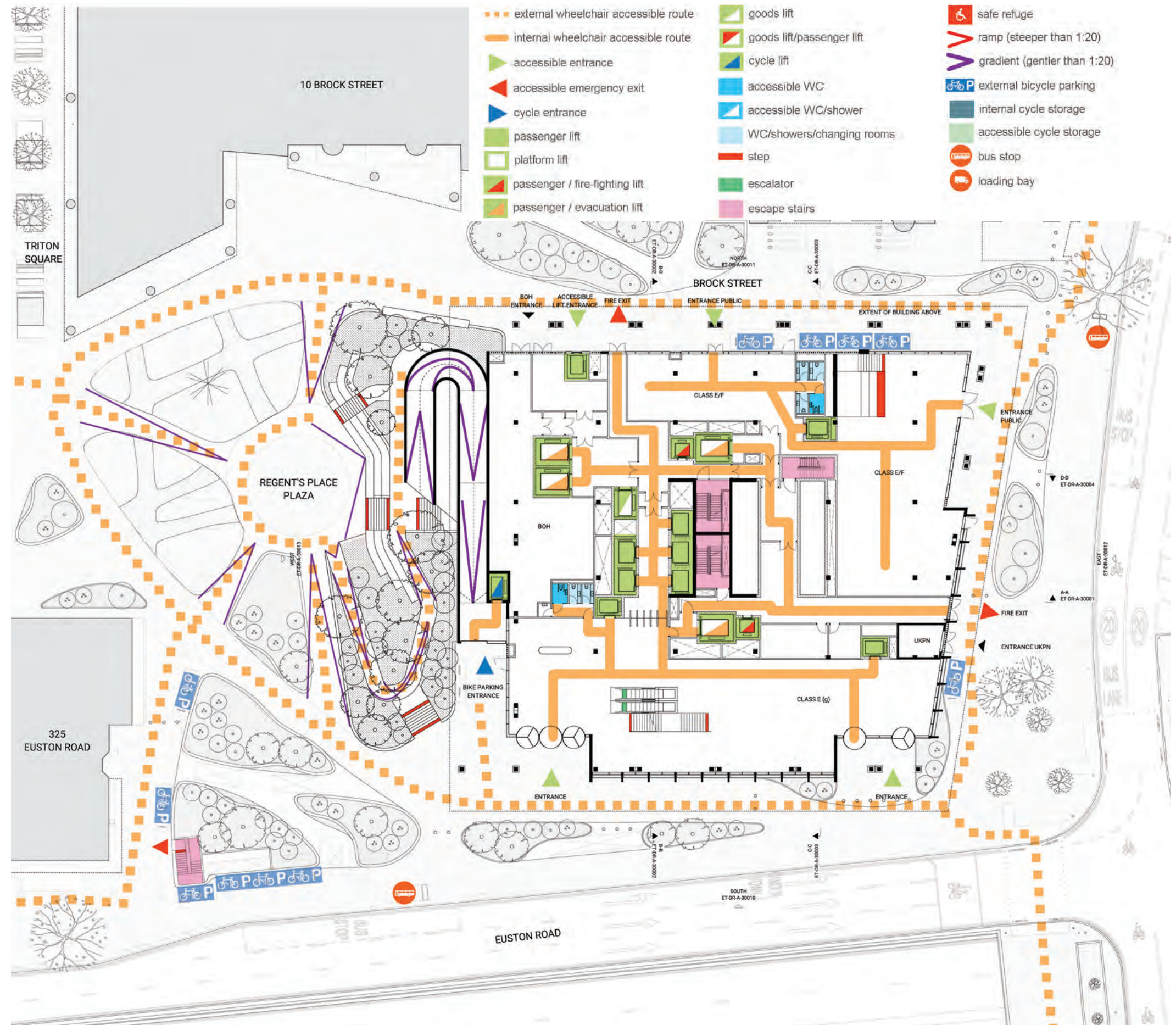
Access Overlay - Ground Floor
